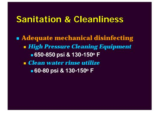
High pressure washing equipment must have adequate force to insure proper cleaning
