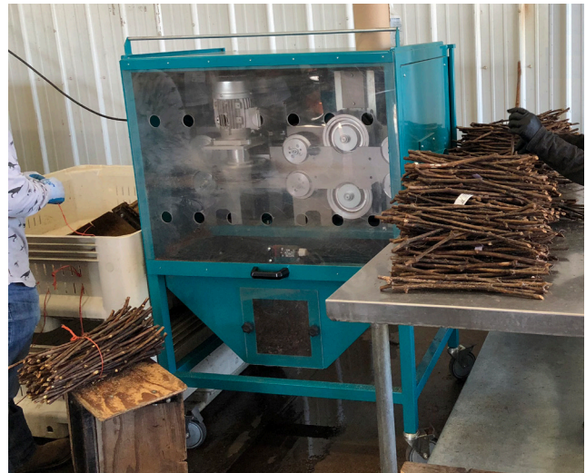
Figure 11. A disbudding machine used to remove buds from rootstock canes.
