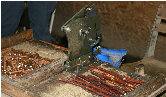
Figure 10. Grafting machine with scion (left side) and rootstock wood (right side).
