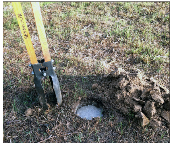
Figure 5. A properly dug hole for a percolation test.
