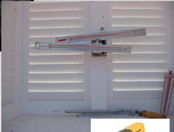
Simple hand-held max/min thermometer—affected by radiation loss
